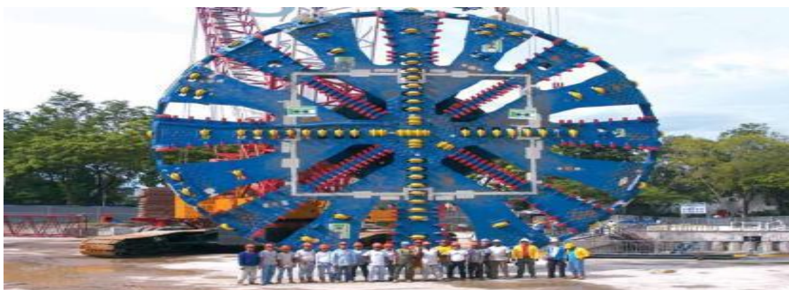
Figure 4: The Slurry Shield TBM at SMART Project Source: DID (2004)
