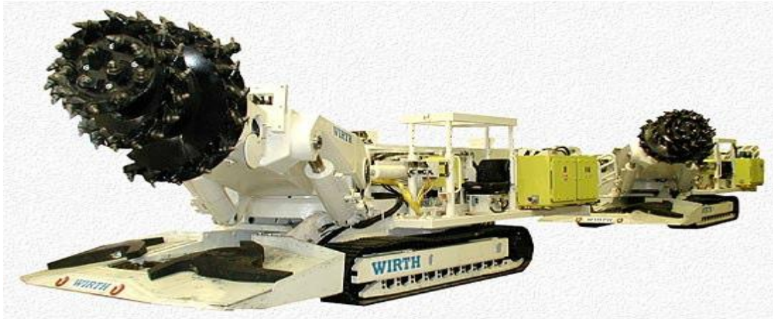
Figure 6: Road Header Machine Source: Mining Technonology.Com (2010)
