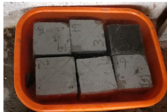
Fig1. Casting of foam concrete cubes
