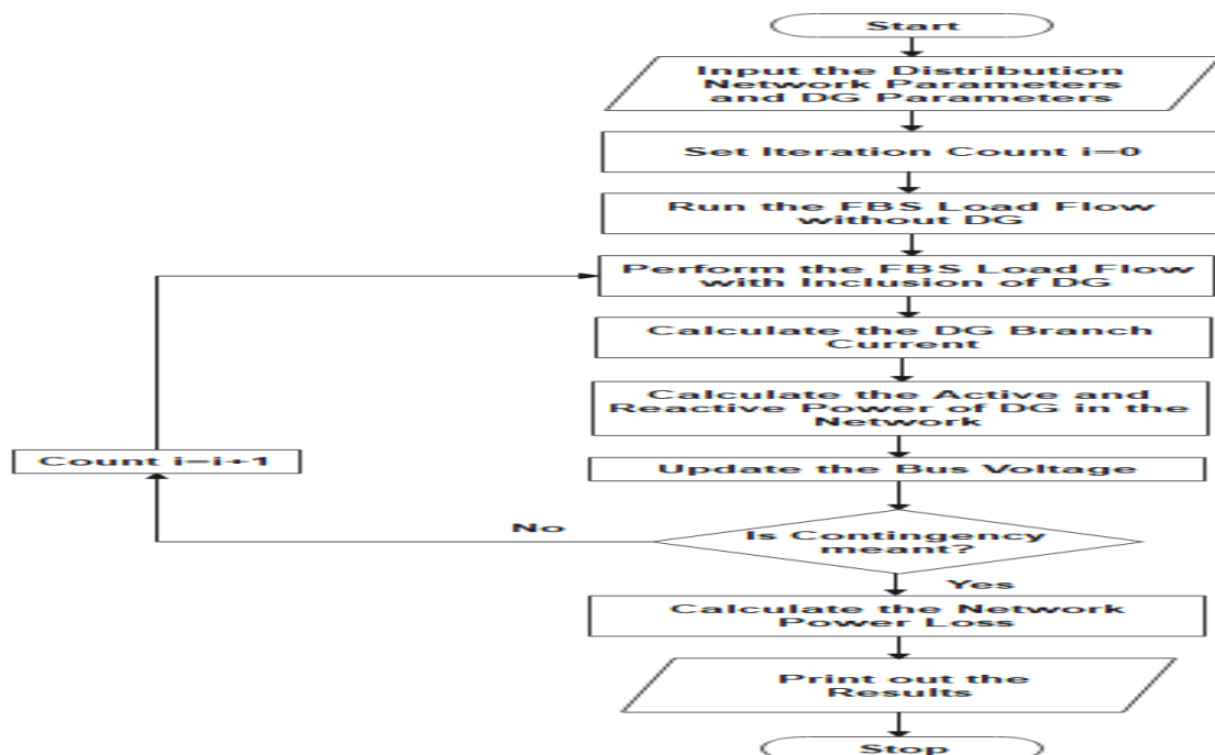
Figure 1b: The Flowchart of Distribution Load Flow without and with DG
