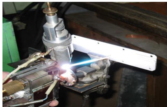
Figure 3. Process of microplasma coating of technically pure aluminum powder METCO 54NS-1 on samples made of titanium alloy OT4
