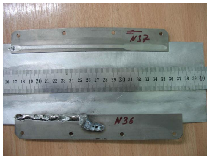
Figure 5. Top view of the sample welded by CO 2 -laser “TR100” at the allowance \Delta=12 mm of titanium alloy OT4 (thickness \delta=1 mm) without coating (upper sample) and with pre-applied coating (lower sample), with aluminum alloy AMg6 (thickness \delta=1.2 mm)
