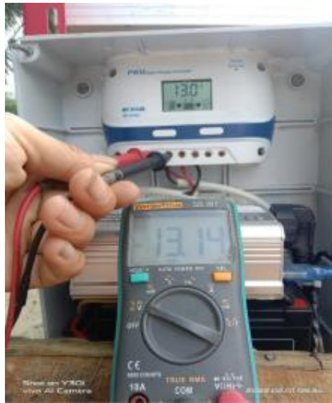
Figure 7. Voltage Measurement Using a Multitester
