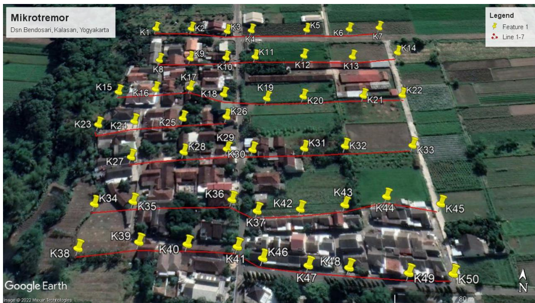
Figure 2. Single Station Microtremor Data Acquisition Survey Design
