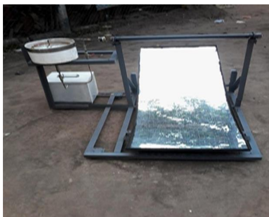
Fig 2.2: Photo plate of the absorption solar refrigerator.
