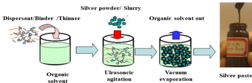
Fig. 1: Preparation procedure of nanoscale silver pastes [9], [32].
