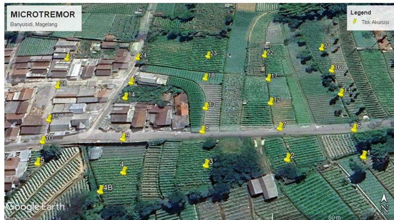
Figure 1. Distribution of microtremor observation stations in Ngepoh Kidul, Banyusidi, Pakis, Magelang. The map and station coordinates are reproduced from the uploaded field summary.
