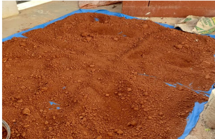
Fig. 6. Homogenized laterite-ash mixture batch, prepared for geotechnical testing.
