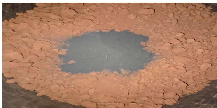
Fig. 5. Incorporation of ash into the lateritic soil during dry mixing (preparation of a test point).
