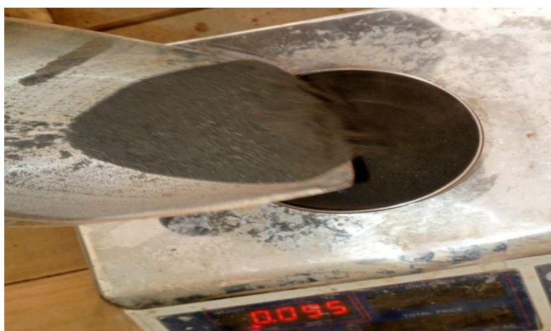
Fig. 4. Weighing of Omni Processor ash during preparation of the laterite-ash mass dosages.
