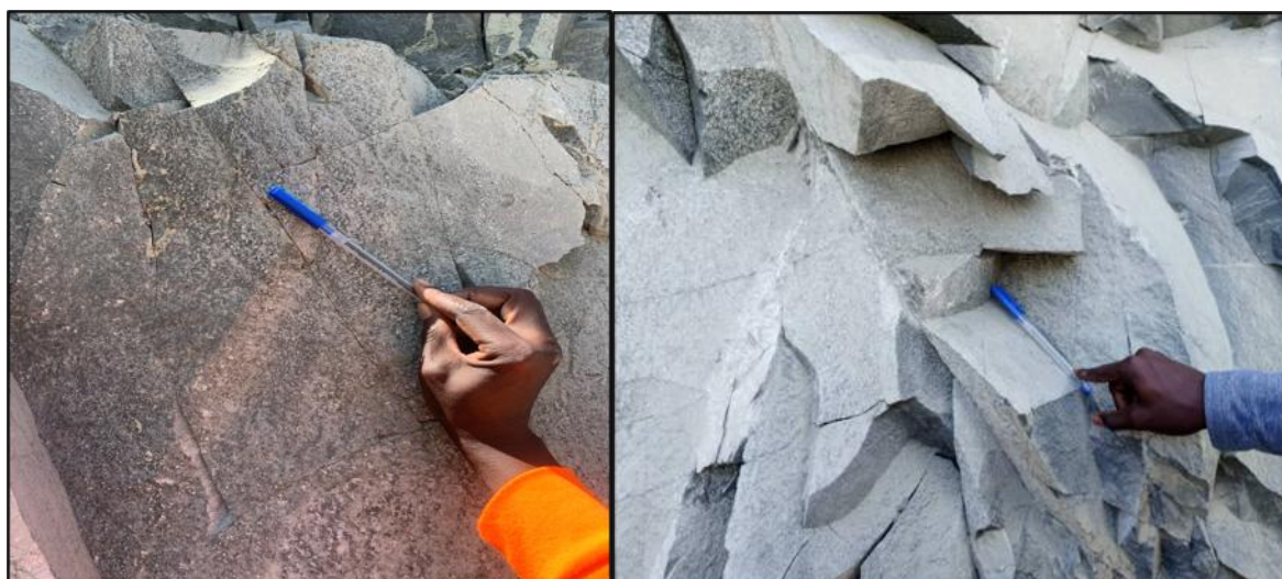
Fig.3: Fracture planes that divide the massif into a polyhedral block
