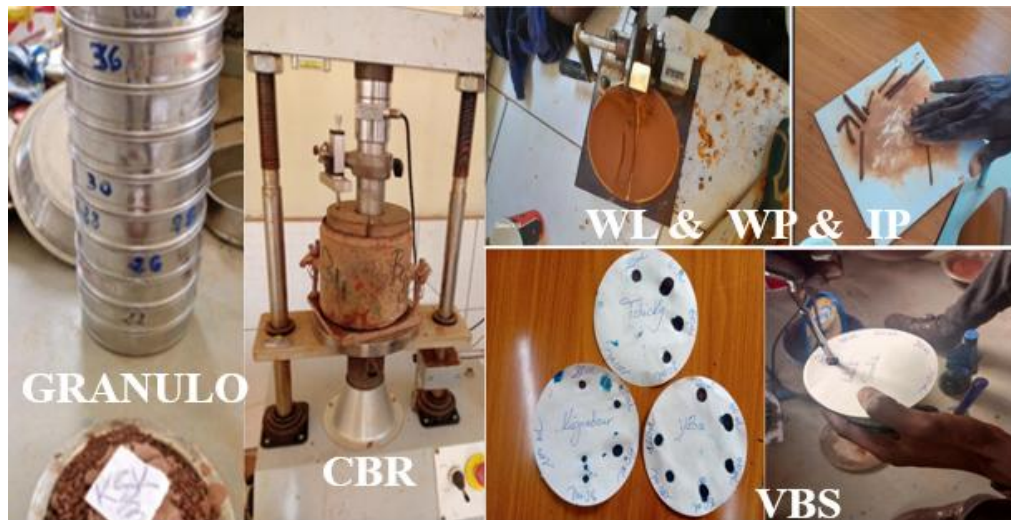
Figure 2 : Various tests conducted in the geotechnical laboratory to identify lateritic materials from quarries
